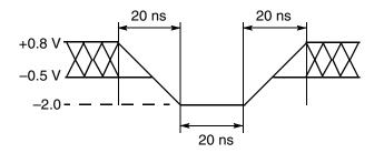
Figure 7. Maximum Negative Overshoot Waveform
