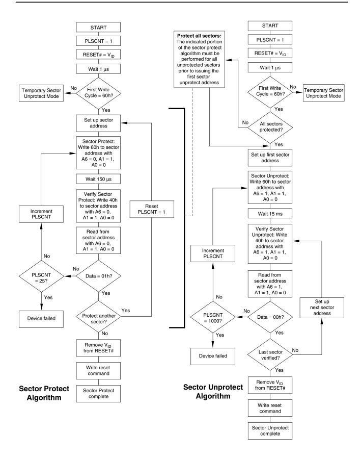
Figure 1. In-System Sector Protect/Unprotect Algorithms
