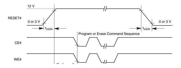
Figure 20. Temporary Sector Unprotect Timing Diagram
