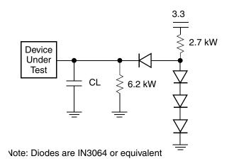
Figure 11. Test Setup
